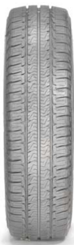
FIG. 1 Front View of the 225/75R16C 116/114S Radial Light Truck Standard Reference Test Tire
