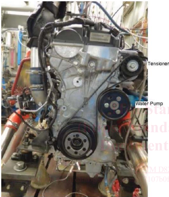
FIG. 3 Water-Pump Drive Arrangement
