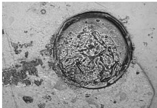
FIG. X1.1 Digital Photograph of Acid Etch Produced During Field Exposure (Jacksonville, FL, 50x-50x magnification)
