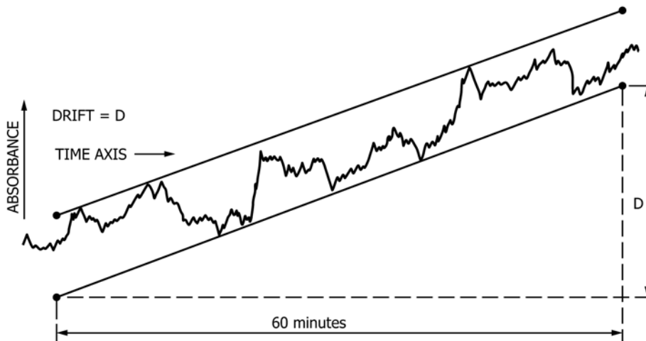
FIG. 2 Example for the Measurement of the Noise and Drift of a VWD (Chart Recorder Output)
