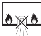
Figure 1 – Symbol for luminaires not suitable for direct mounting on normally flammable surfaces (suitable only for mounting on non-combustible surfaces)
