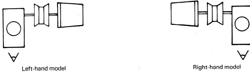
Figure 2 – Type 2 – Single cable-lifter windlass, fully powered
