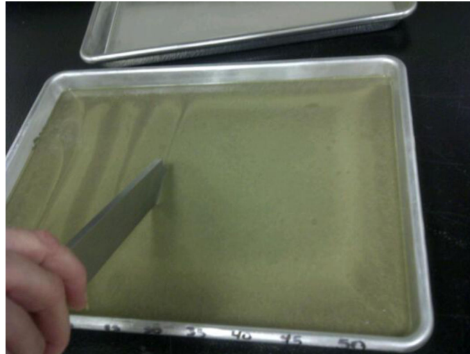
FIG. 1 Full-Depth Cut in Test Specimen
