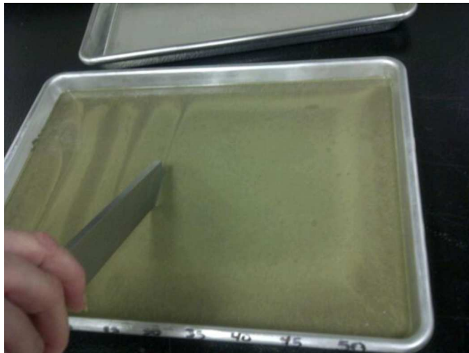
FIG. 1 Full-Depth Cut in Test Specimen
