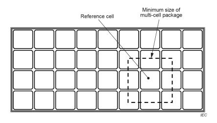
Figure 2 – Single reference cell in a multi-cell package
