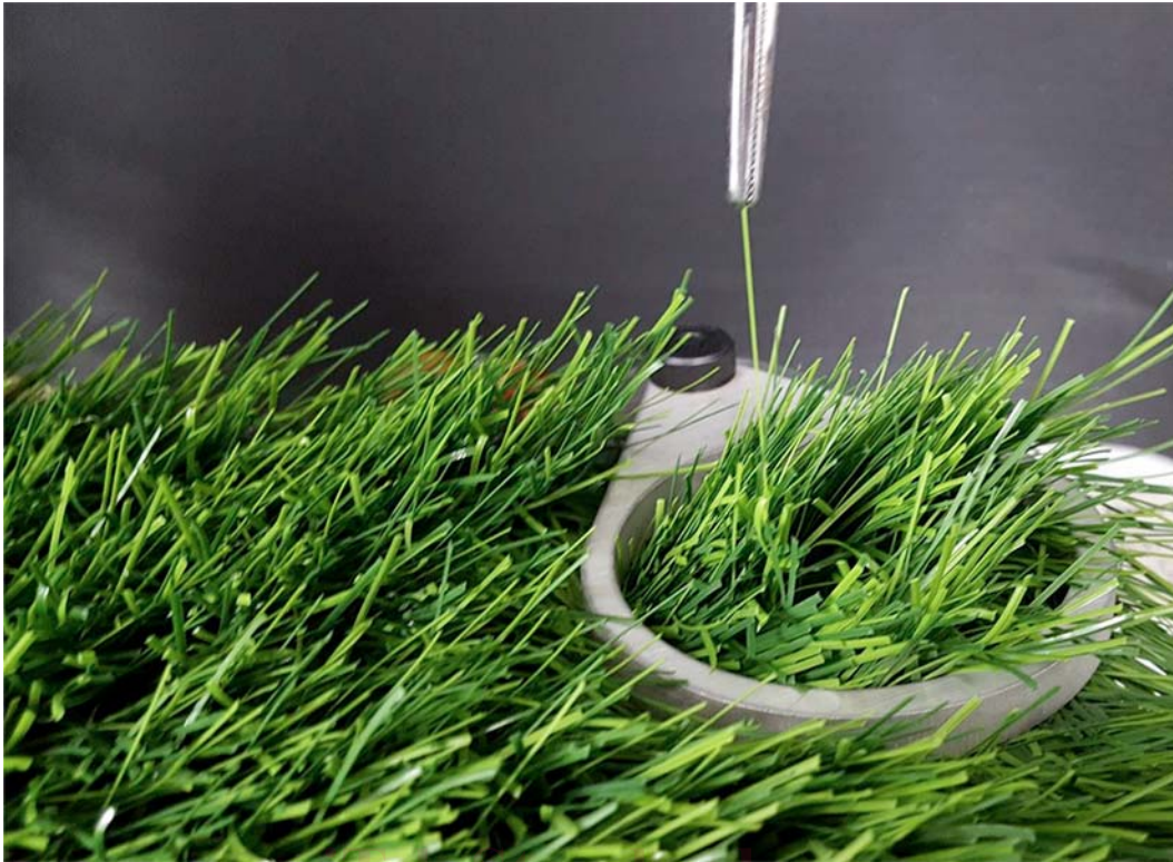
FIG. 5 Single Filament in Filament Clamp
