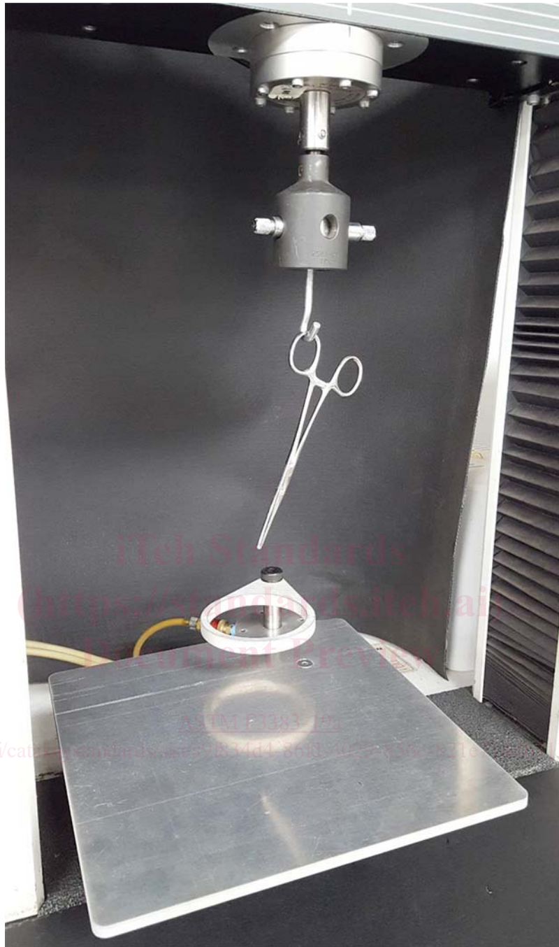
FIG. 2 Example of Sample Clamp (Pneumatic)
