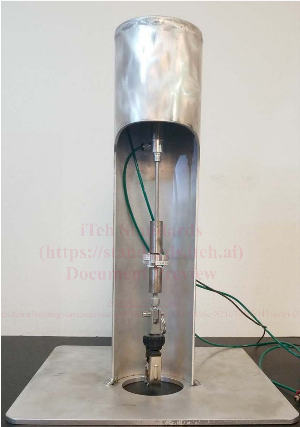
FIG. 7 Example of Portable CRE Type Device
