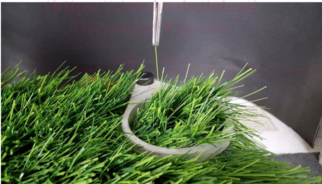
FIG. 6 Direction of Pull for Filament Bind
