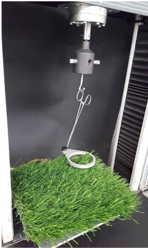
FIG. 3 Test Sample on Platen
