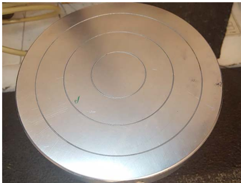
FIG. 1 Example of Flat Platen
