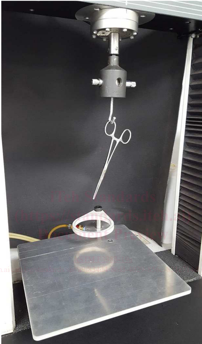
FIG. 2 Example of Sample Clamp (Pneumatic)
