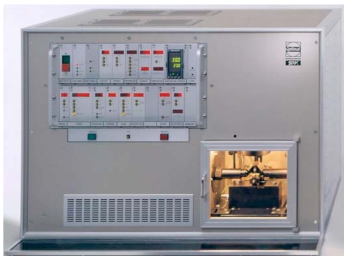
FIG. 1 SRV Test Machine (Model III)
