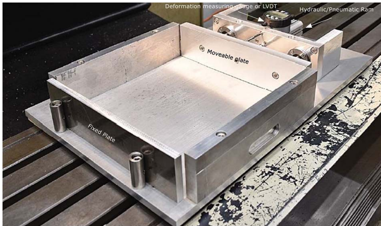
FIG. 1 Mold System That Can Control Lateral Pressure on Two Opposite Sides of Slab Specimen
