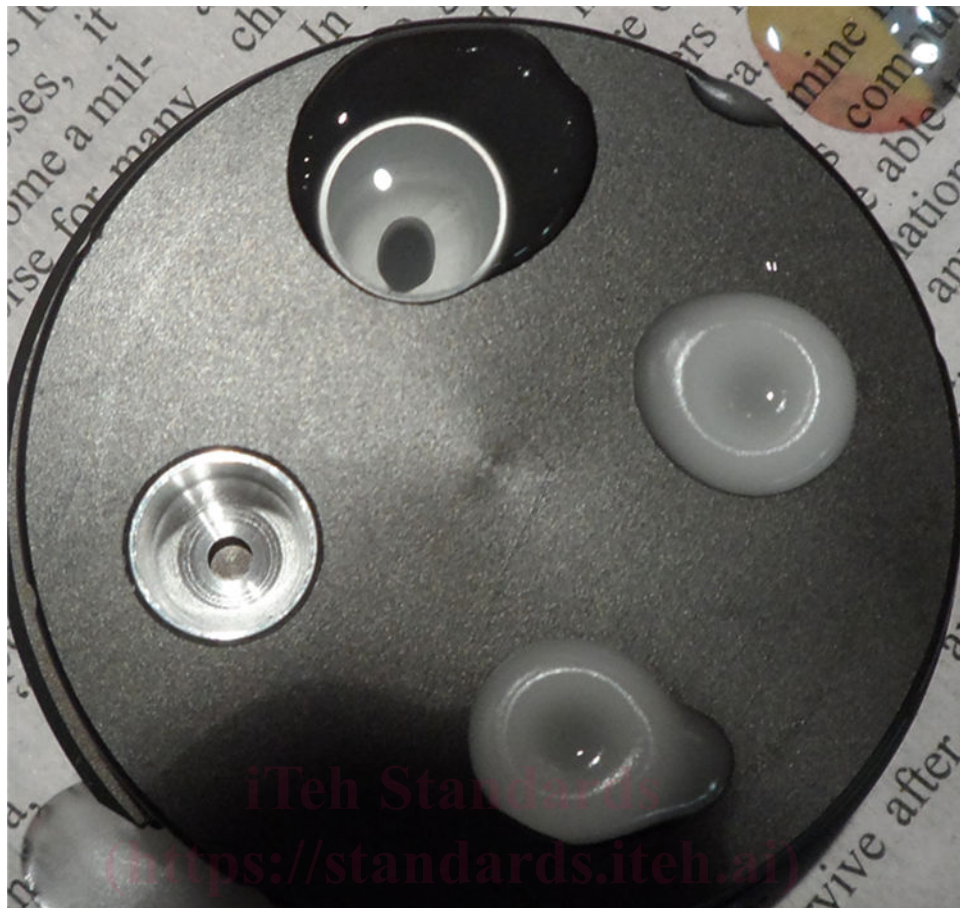
FIG. 2 Four Recently Poured Dropping Point Cups
