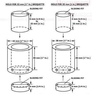
NOTE 1—Material: cold rolled or stainless steel. Dimensions *a* and *b* (inside diameters) are nominally 32 mm  $[1^{1/4} \text{ in.}]$  and 25 mm [1 in.]. If an automatic polishing attachment is to be used, these dimensions should be specified to yield a briquet fitting snugly in the briquet holder.
