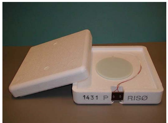
FIG. 1 Example of a polystyrene calorimeter used for routine measurements at a 10-MeV industrial electron accelerator
