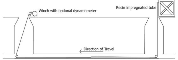
The resin impregnated tube is pulled into place using a winch. A slip sheet is placed in the bottom of the pipe prior to this process.
