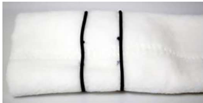
FIG. 1 SMHG O-Rings on Lateral Tube
