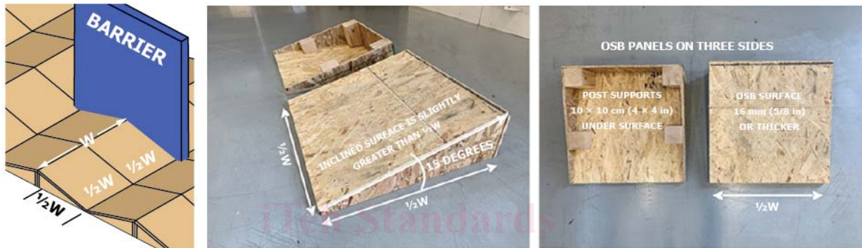
FIG. 6 Details of a Pitch/Roll Ramp
