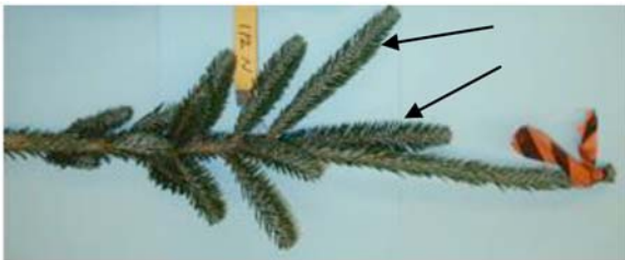
FIG. 3 A 2-year-old Branch Specimen with Arrows Showing a Pair of Current-Season Shoots to be used for Moisture Content and Fire Tests
