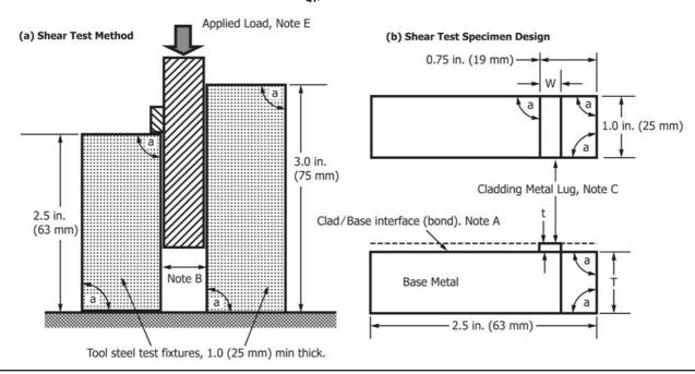
Note 1—The cladding metal shall be removed (machined) from the base metal over the full interface surface except for the area of the clad metal test lug. The machined surface shall lie within  $\pm 0.001$  in. (0.05 mm) of the interface (bondzone). If the bond has a wave morphology, the interface shall be defined as the centerline of the wave height.
