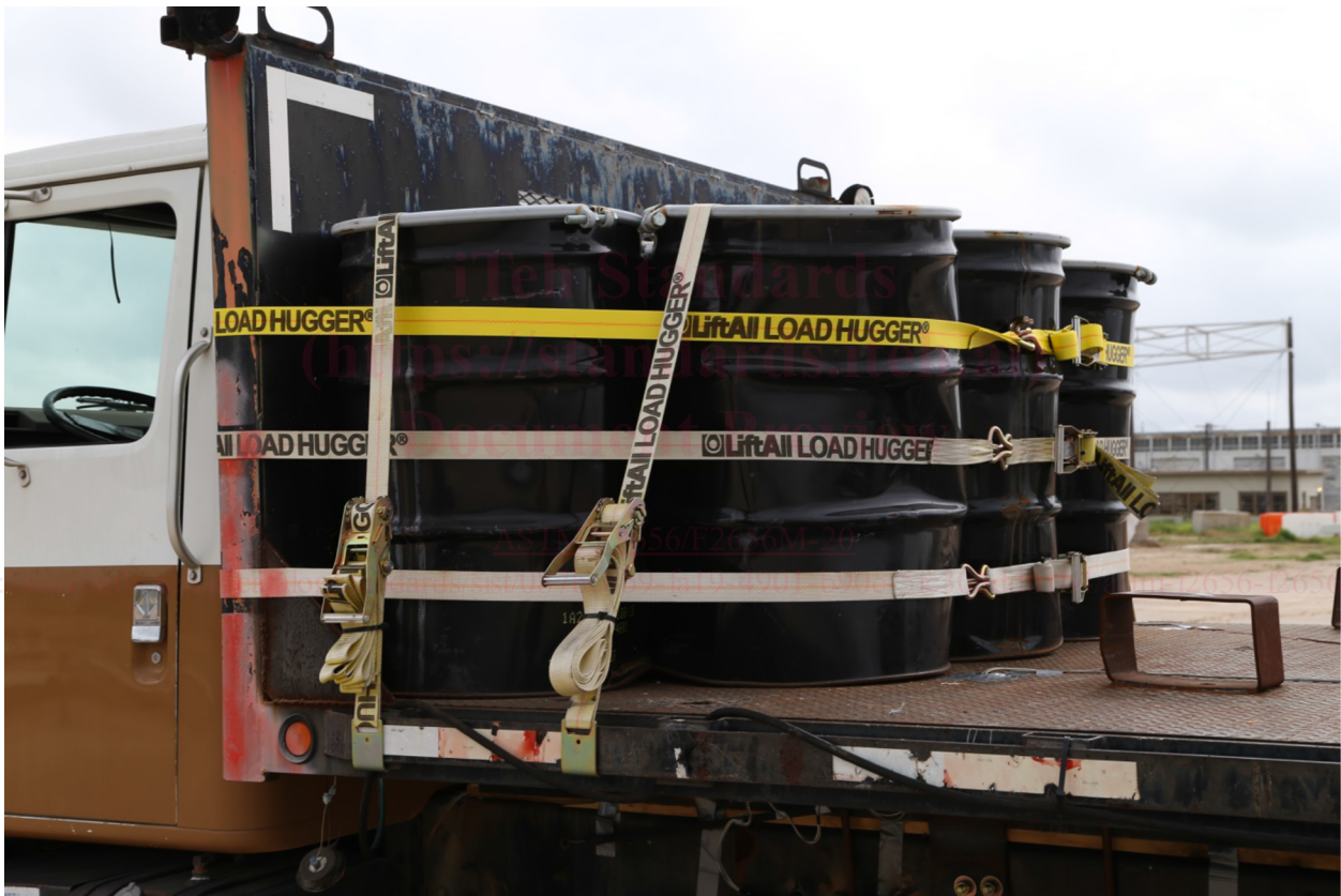
FIG. 2 Typical Ballast Attachment, Rear View
