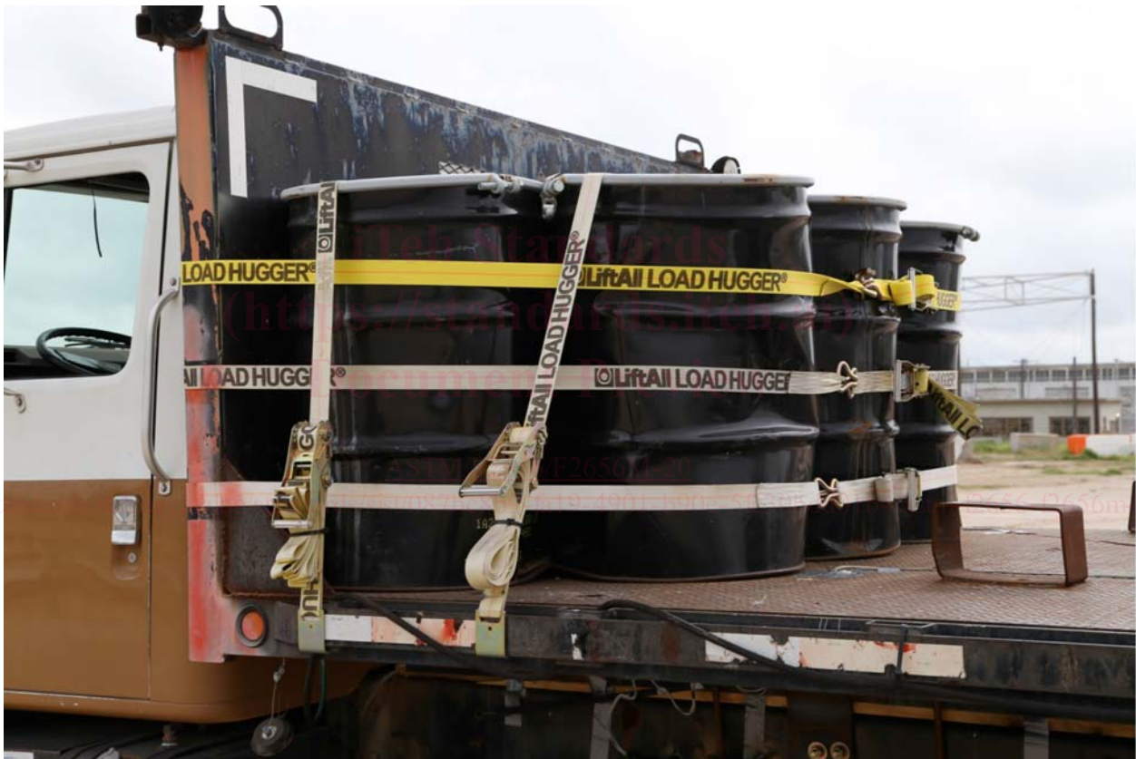
FIG. 2 Typical Ballast Attachment, Rear View
