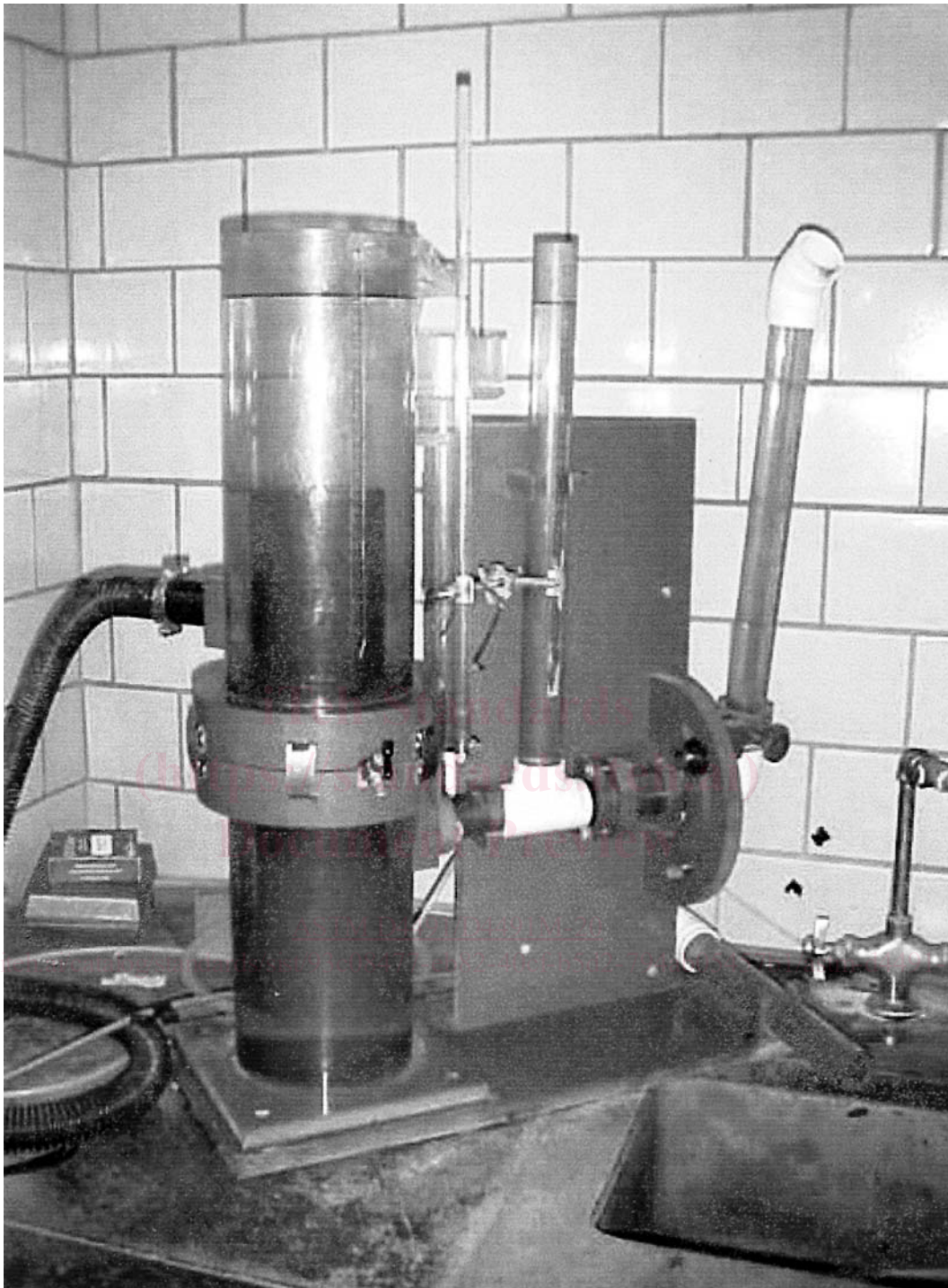
FIG. 1 Constant and Falling Head Permeability Apparatus
