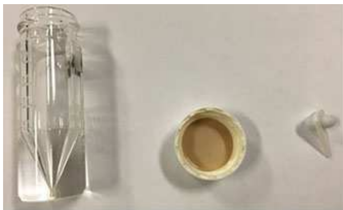
FIG. 1 Micro Reaction Vial with PTFE Lined Cap and Triangular Magnetic Stirring Bar
