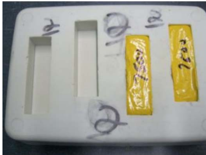
FIG. 4 Silicone Mold with Cooled Samples
