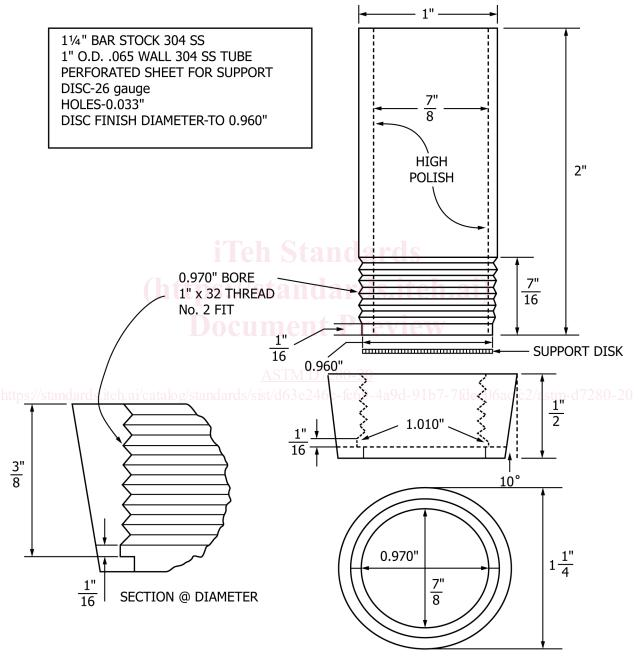
FIG. 1 Stainless Steel Filtering Crucible with Support Disk
