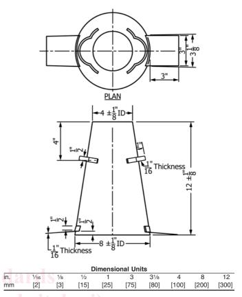
FIG. 1 Mold for Slump Test
