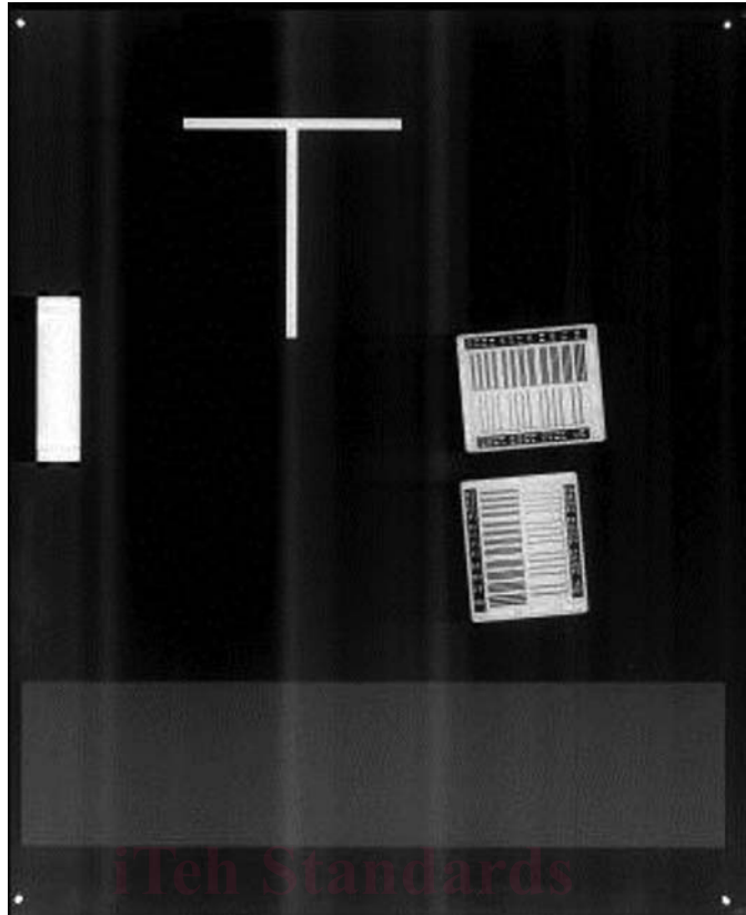
FIG. 2 Example of Banding (Parallel to IP Transport Direction) in a Computed Radiograph of a Prototype Test Phantom
