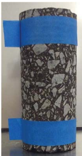
FIG. 5 Example Restrained Specimen Prepared for Gluing
