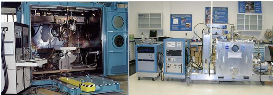
FIG. 5 Ground-based (Left) and Portable (Right) Electron-Beam Freeform Fabrication Systems (Courtesy of NASA Langley Research Center)
