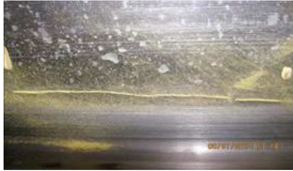
FIG. 34 Two Cracks on a Tooth Just Above the Root That Were Only Observed Visually After Being Revealed by the ECA Examination; In This Example, the Cracks Were Not Apparent Visually Until MT Was Performed
