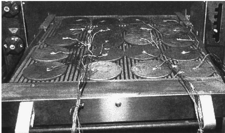
FIG. 2 Thermocouple Disk Placement
