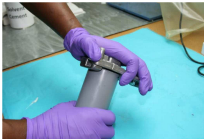
FIG. 7 Debur and Chamfer the Pipe End
