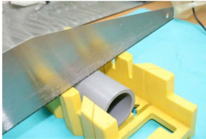
FIG. 5 Cut the pipe straight at a 90° angle.
