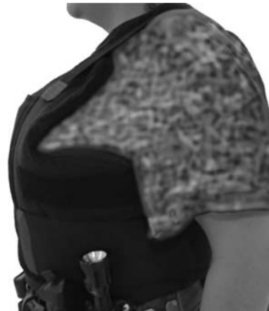
FIG. 6 Example Armor Showing Lack of Continuous Coverage
