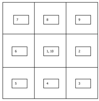
Note 1—A sequence of nine, non-overlapping measurements which will reveal side-to-side, center to edge, and top to bottom non-uniformities of luminance. The order of sampling is suggested by the numbers. See 5.8.
