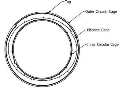
NOTE 1—The total reinforcement area of the inner circular cage and the elliptical cage shall not be less than that specified for the inner cage in Tables 1-5.
