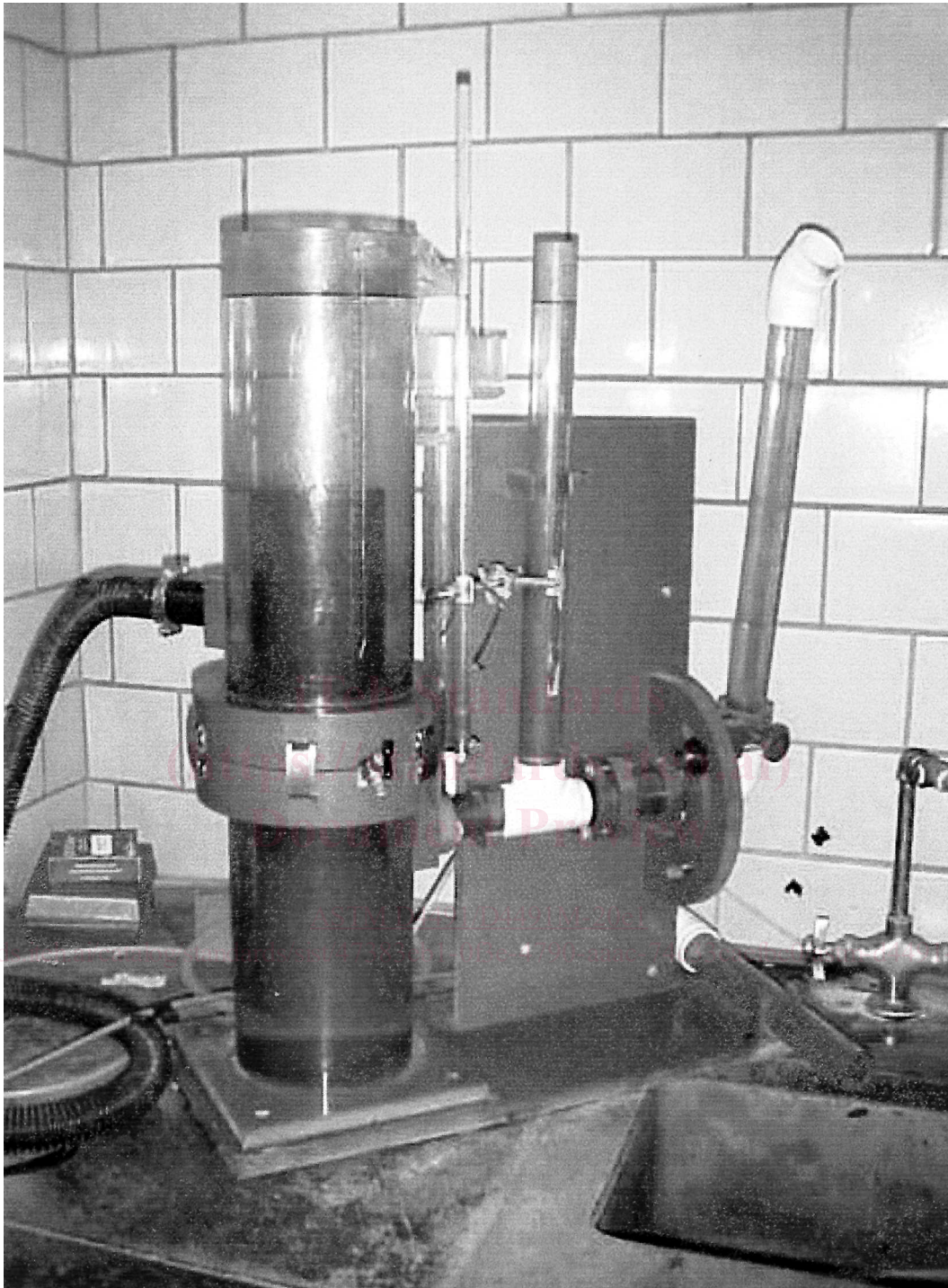
FIG. 1 Constant and Falling Head Permeability Apparatus
