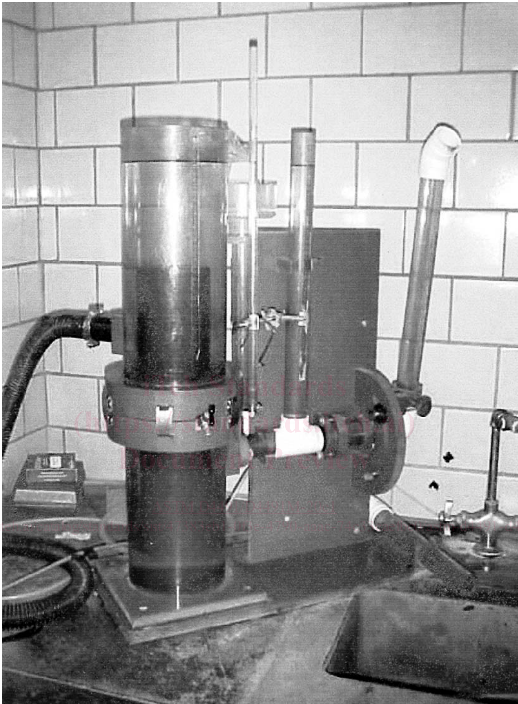
FIG. 1 Constant and Falling Head Permeability Apparatus
