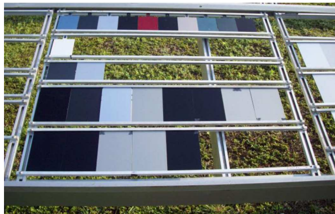
FIG. 1 Suitably Mounted Specimens in a Frame
