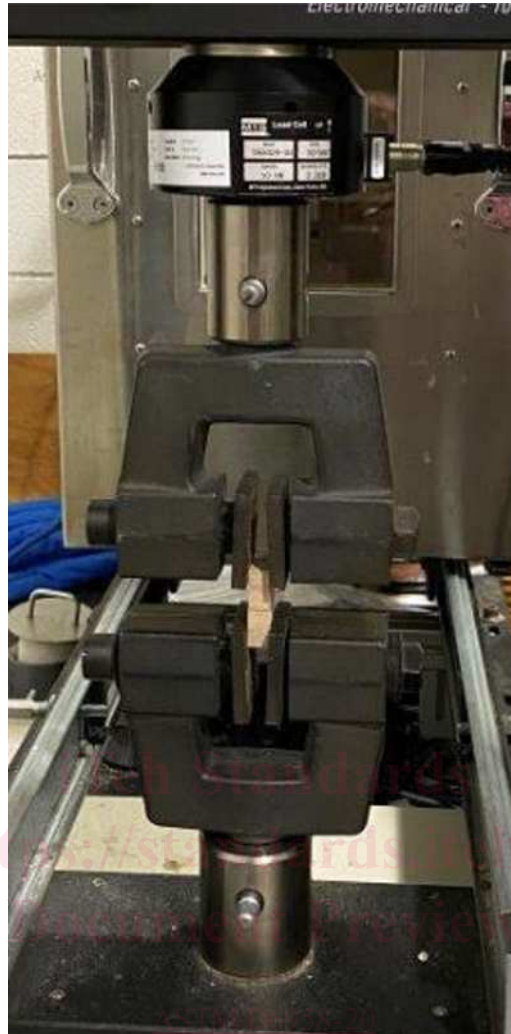
https://standards.iteh.ai/catalog/standards/sist/5-638f802b19e8/astm-d6958-20 FIG. 2 Assembly Secured in Testing Machine
