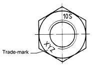
The marking shall be indented on either the top or bottom face of chamfered nuts and shall be either indented or embossed on
