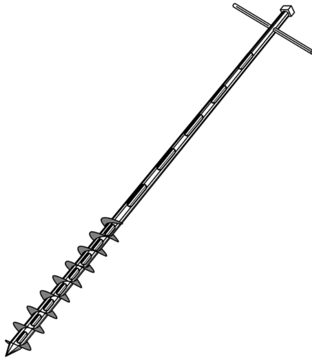
FIG. 2 Multi-Level Slot Sampler with Auger Point (Keystone Sampler)
