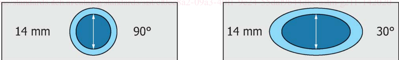
FIG. 5 Erosion Scar Size Recommended by Adjusting Nozzle to Coupon Standoff Distance with 25 mm by 75 mm Type 410 Stainless Steel Test Specimens
