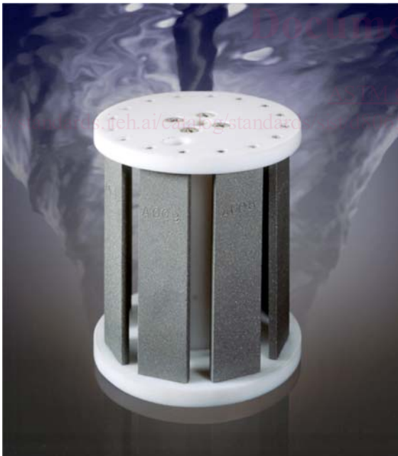
FIG. 2 Photo of Rotating Cage Containing Coupons
