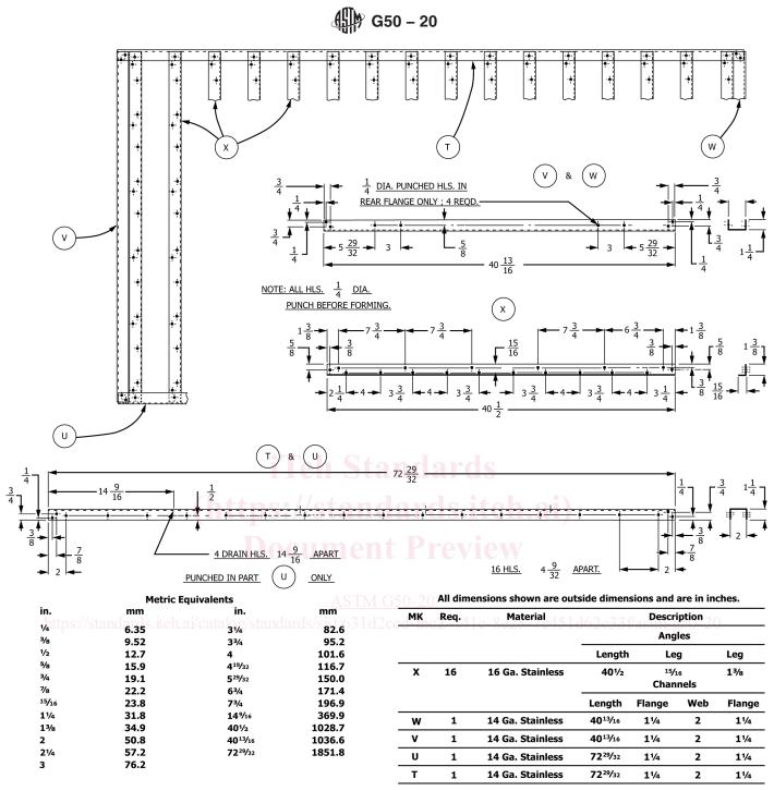
FIG. 1 Suitable Test Frame
