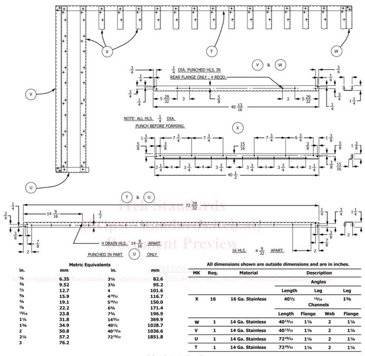
FIG. 1 Suitable Test Frame
