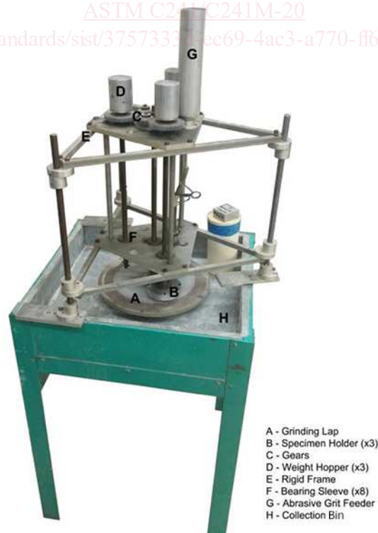
FIG. 1 Apparatus for Abrasion Resistance Test of Stone
