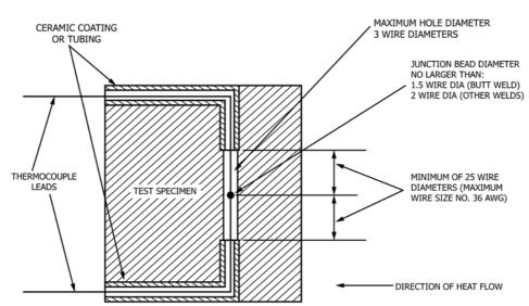
Note 1—If a number of thermocouples in depth are required, drill holes at varying locations on the circumference.
