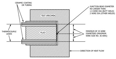
Note 1—Plug and test specimen of same material.
